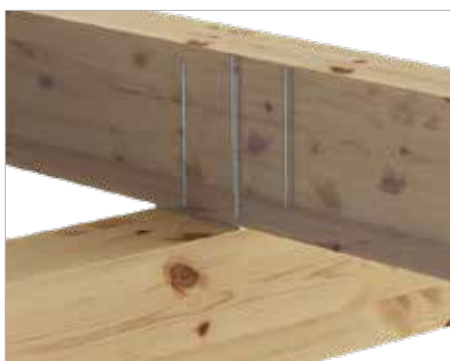
Reinforcement in the point of support
