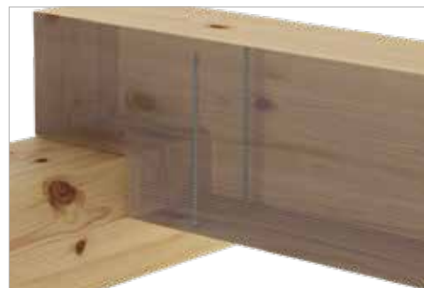
Protection against failure of notched beam
