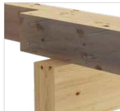
Joint between two passing-by beams
