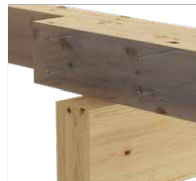
Joint between two passing-by beams
