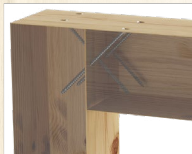
Joint between two girders
