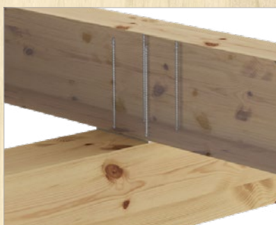
Reinforcement in the point of support
